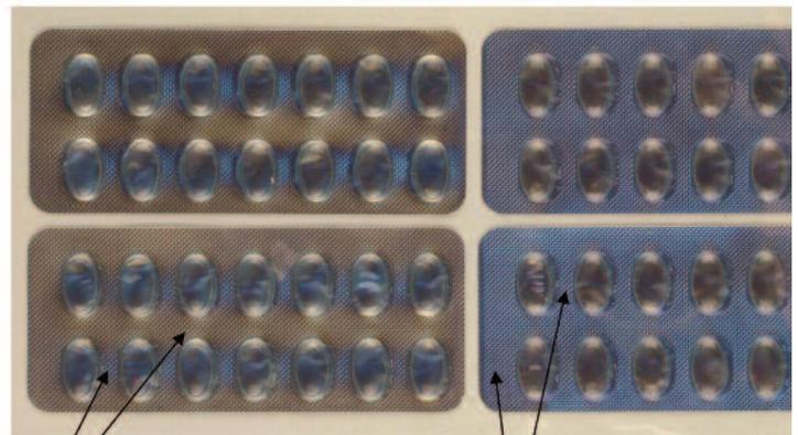
Color differential in the sealed area is an indication of stress-forming. Relaxation can cause micro-channeling
